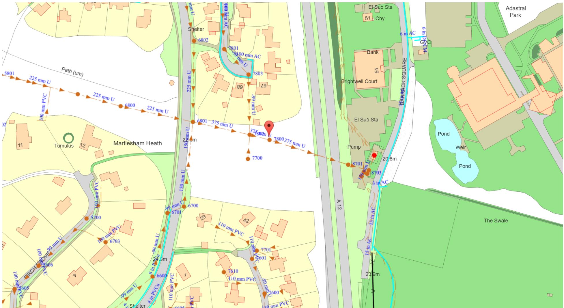
**Figure 3: Showing your water recycling Foul Water point of connection**
